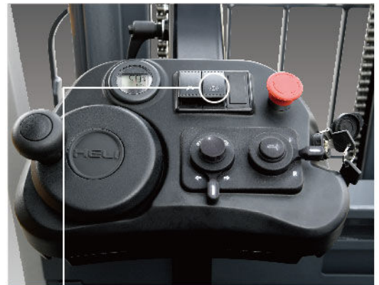
The electronic parking brake system (EPB) realizes one button parking brake and it is convenient and comfortable to operate.
