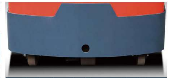
Standard auxiliary wheel, higher truck stability
